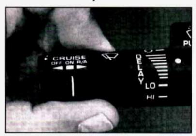
You control the windshield wipers by turning the band with the wiper symbol on it.
